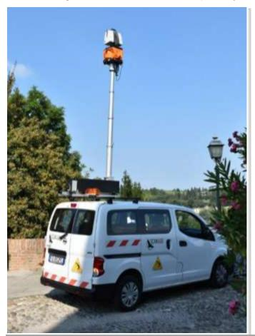
By using Level-Lift Roof combined with Level-Plane 16 and raising the 3D Laser Scanner gripping point it's possible to obtain:
